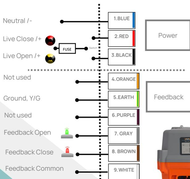
Remove wiring box via 4 x screws. This will expose the wiring terminal. Simply match the colours and codes you see against the above. Then re fit the wiring box and ensure seal is in place.
