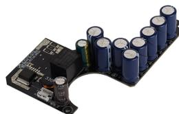
Failsafe via internal super capacitor if you have selected Failsafe version. Capacitor is charged whilst power applied. When power is removed capacitor will close/open actuator.
