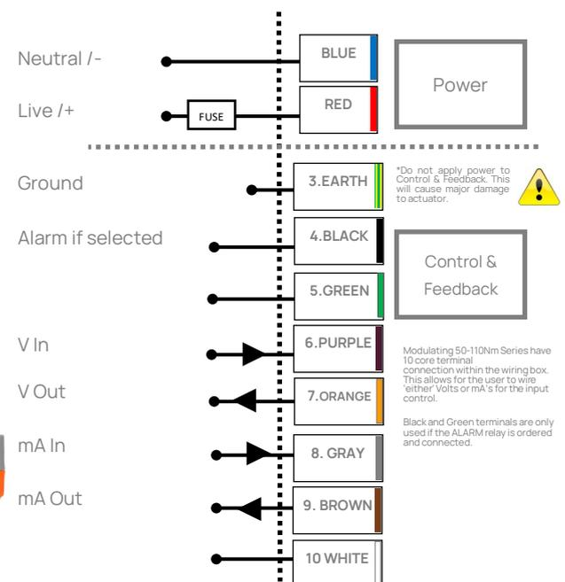
\*Do not apply power to Control & Feedback. This will cause major damage to actuator.
