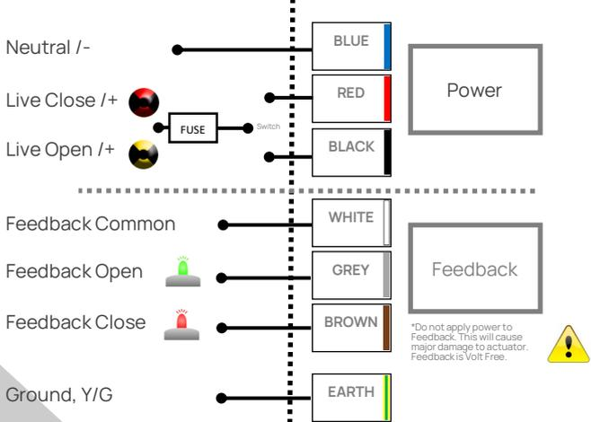
\*Do not apply power to Feedback. This will cause major damage to actuator. Feedback is Volt Free.
