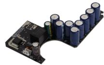
\*Failsafe via internal super capacitor
