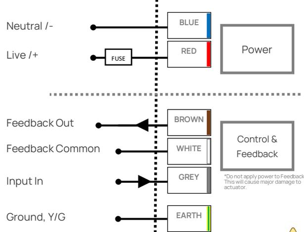
\*Do not apply power to Feedback. This will cause major damage to actuator.
