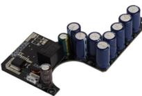
\*Failsafe via internal super capacitor
